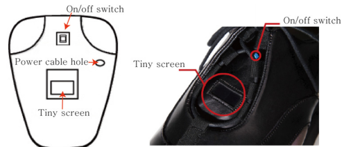
Figure 4. The interface of the battery display on the shoe Tongue.
