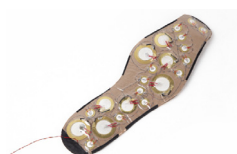
Figure 9. Developed double-layered piezo insole (left side).
